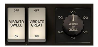
The Vibrato and Chorus in a vintage tonewheel organ is not like the vibrato or chorus effects in guitar amps or stomp boxes. Tonewheel organs included a unique and somewhat complex "scanner vibrato" circuit that's been super accurately simulated in Blue3.
